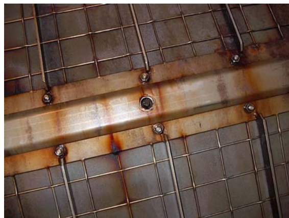
Fig. 10. Detail of nuts and bolts of rotating screens.
